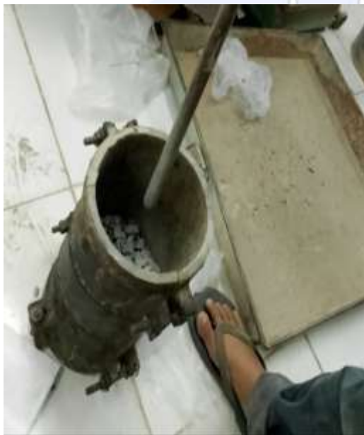
Proses penumbukan 25 kali perlapisan
