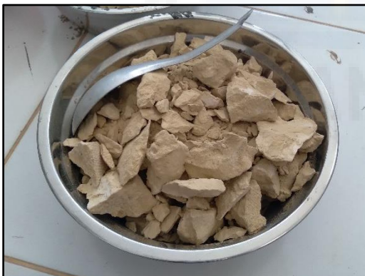
Gambar K.5 Bongkahan FGD-Gypsum
