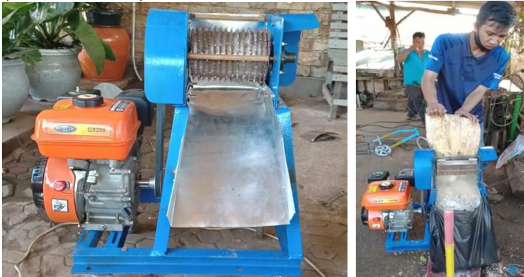
Gambar 3. Mesin parut sagu (Achmad, 2020)
