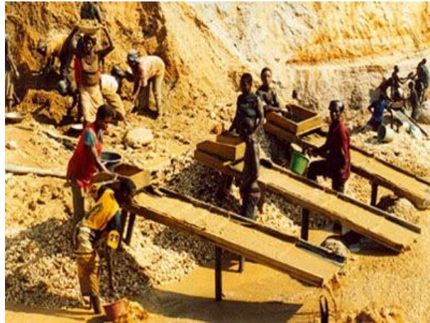
Gambar 2.6 Metode manual ( manual mining method )
