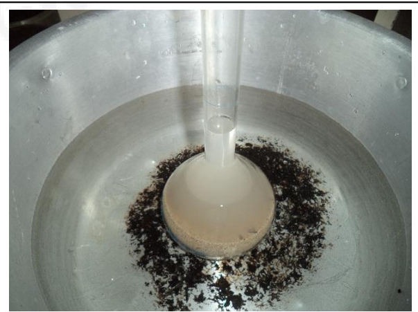
Gambar. Pasir Pantai Keadaan SSD
