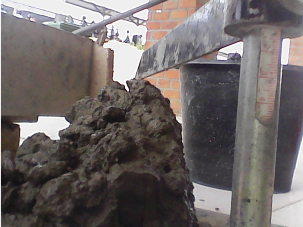
Gambar L.D.19 Pengujian Nilai Slump Test
