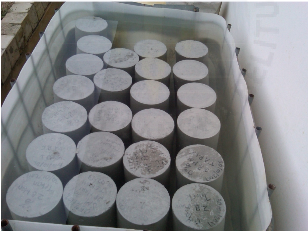
Gambar L.D.22 Proses Perawatan Beton
