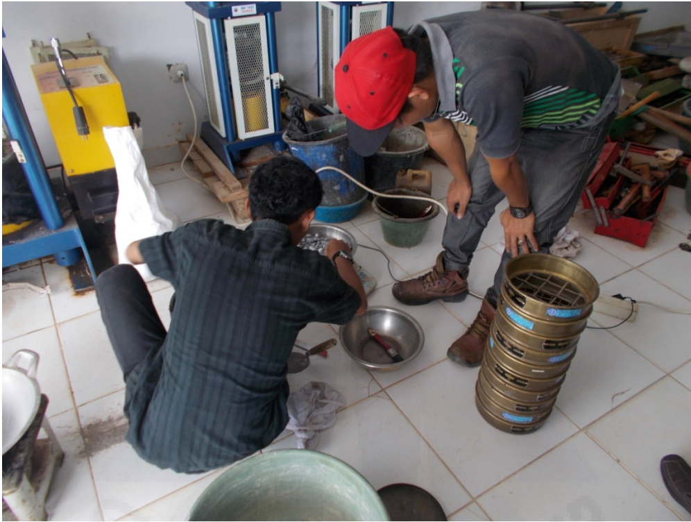
Gambar L.D.7 Proses Penimbangan Lolos Saringan Agregat
