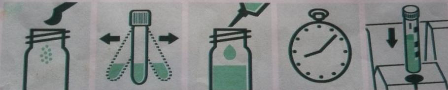
**Add** 1 level blue micro-spoon of  $\text{NO}_3\text{-1K}$  into a reaction cell and close with the screw cap.
