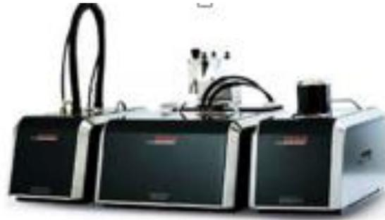
**Gambar 2.9** PSA (*Particle Size Analyzer*) (Lusi, 2011)
