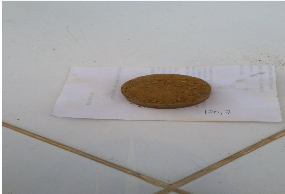
Bahan uji Direct Shear
